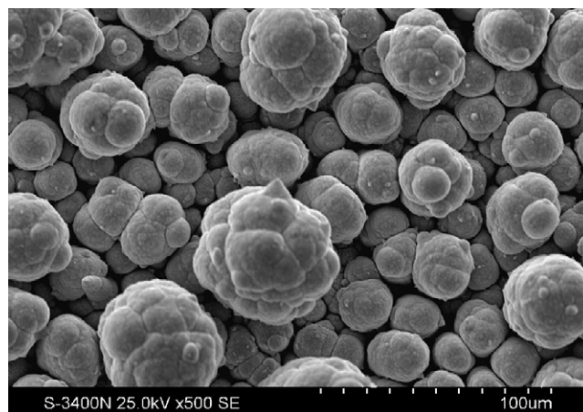
Fig. 4. SEM image of copper coating on steel.
